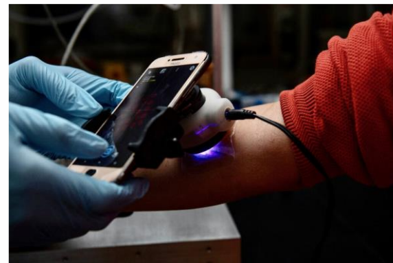
Wearable skin patch sensors (smart dressing) for metabolites monitoring by smartphones
